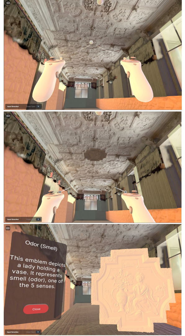
Figure 9: VR LOD System. Users can navigate and interact with patterns on the 3DGS ceiling (top). When a pattern is selected, the aligned emblem mesh appears (middle), triggering an animation that brings it into the near-eye field for detailed viewing accompanied by storytelling elements (bottom).
