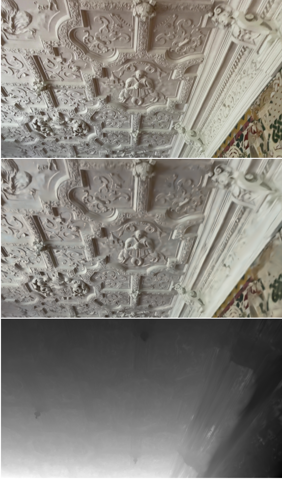
Figure 6: View (middle) and depth (bottom) renderings from 3D Gaussian Splatting trained by depth-regularized framework. PSNR: 22.16 dB, SSIM: 0.7015, LPIPS: 0.5427 against evaluation frame (top).
