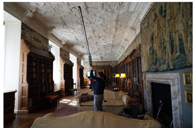
Figure 4: 3D Scanning of features in the ceiling of the Long Gallery in Blickling Hall. An Artec Eva is attached to an extended telescopic tripod to get the scanner within 0.4 to 1m range of the ceiling and it is scanned whilst viewing the capture area on a laptop. This is achieved with two people to ensure free movement of scanner and laptop whilst capturing.
